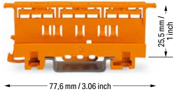
Mounting carrier; for 2-, 3- and 5-wire splicing connectors (4 mm 2 ); 17.5 mm wide
