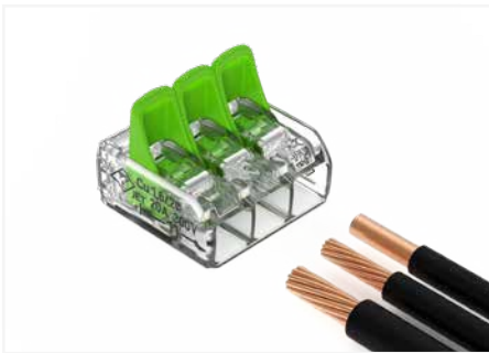
4 mm 2 : Tool-free connection of up to 10 stripped, fine-stranded conductors from 0.14 ... 4 mm 2 , as well as solid or stranded conductors from 0.2 ... 4 mm 2 (24 ... 12 AWG). 6 mm 2 : Tool-free connection of up to five stripped, fine-stranded as well as solid or stranded conductors from 0.5 ... 6 mm 2 (20 ... 10 AWG).
