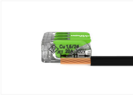
4 mm 2 : Strip conductor to 11 mm (0.43 inch). 6 mm 2 : Strip conductor to 12 ... 14 mm (0.47 ... 0.55 inch).
