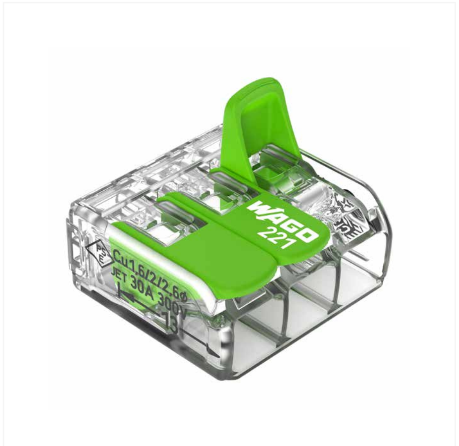
4 mm 2 : Tool-free connection of up to 10 stripped, fine-stranded conductors from 0.14 ... 4 mm 2 , as well as solid or stranded conductors from 0.2 ... 4 mm 2 (24 ... 12 AWG). 6 mm 2 : Tool-free connection of up to five stripped, fine-stranded as well as solid or stranded conductors from 0.5 ... 6 mm 2 (20 ... 10 AWG).
