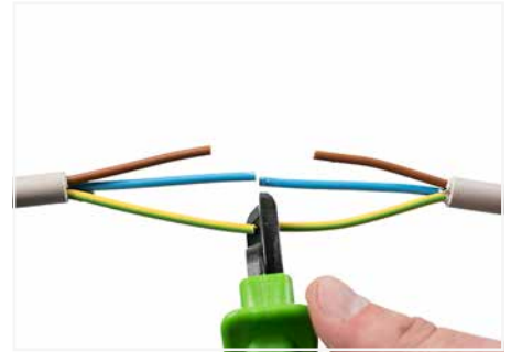
Cut out the damaged areas in the copper and disconnect all other conductors. For damaged areas between 1 mm and 30 mm, at least 30 mm of the damaged conductor must be removed. Tip: A connector (approx. 30 mm long) can be used as a length guide.
