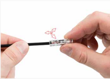
Twist the connector alternately left and right while pulling it off the conductor.
